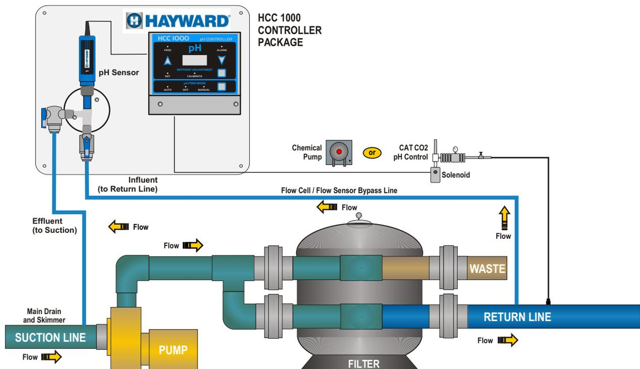
ALL CHEMICALS MUST BE INJECTED DOWN STREAM FROM HEATER & FLOW CELL
