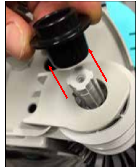
Step 3: Remove Roller bushing from Roller Wheel Shaft.
