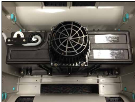
Filter Bucket Housing removed
