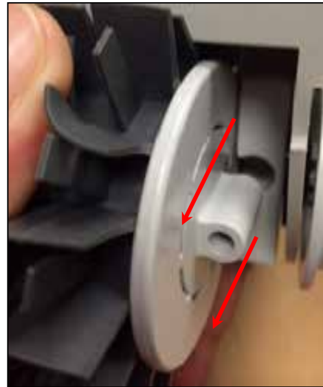
Step 2: Carefully pull wheel tube away from wheel axles.
