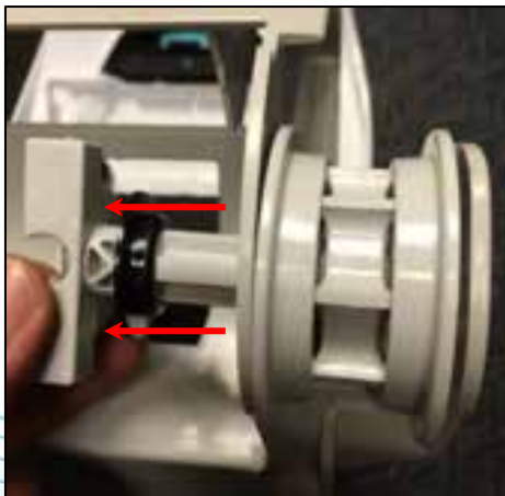
Step 1: Unscrew T20 screw from each side of roller.
