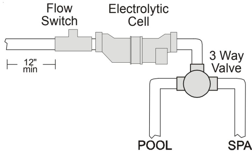
The cell may be mounted vertically or horizontally, and water can move in either direction through the cell. Install using the 2" unions provided. Tighten unions **BY HAND** for a watertight seal. For systems with 1½" plumbing use adaptors (provided by installer).
