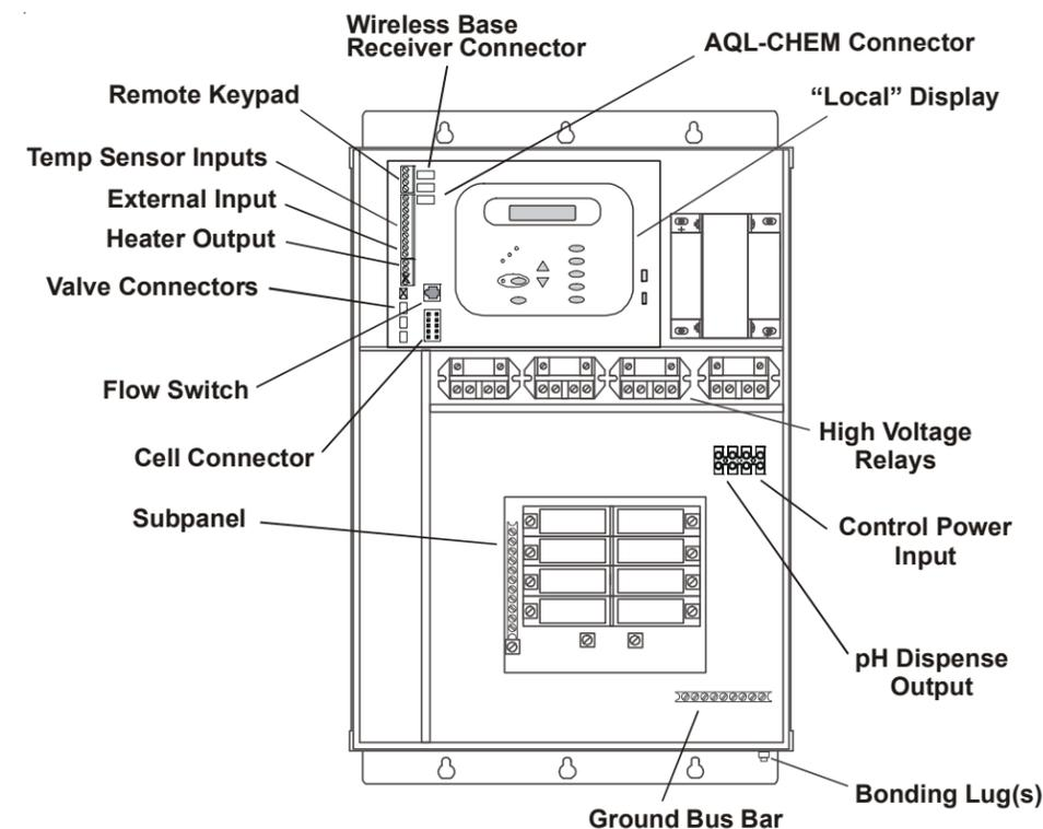
The Pro Logic Control Center requires both high and low voltage connections. Low voltage connections will be made to actuators, sensors, remote keypad, etc. High voltage connections will be made to pumps, lights, etc., as well as providing direct input power to the Control Center. Always:
