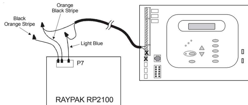
*Drawing is for digital heater. If heater is a millivolt (analog), run red wires from Fireman's Switch to heater relay.*
