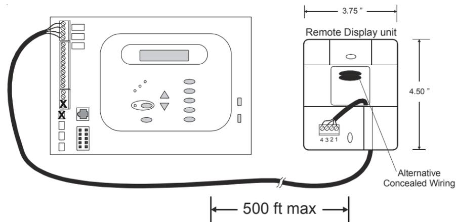
*If multiple remote display/keypads are installed:* Never connect more than 2 wires to any terminal block. Two remotes can be wired back to the Pro Logic main unit or the second display/keypad (and third, if applicable) can be "daisy chained" with one display/keypad wired to the next. The maximum wire run from the Pro Logic main unit to the furthest remote display/keypad is 500 ft (160m).
