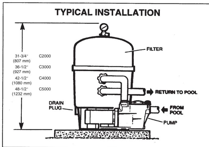
**NOTE: If rigid piping is used, installation of a piping union is recommended for ease of future servicing.**
