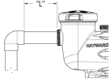
**\* Note:** It is recommended that a minimum length of straight piping (shown as "L" in above diagram), equivalent to 5 pipe size diameters, be used between the pump suction inlet and any plumbing fittings (elbows, valves, etc.).
