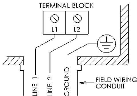
**ATTENTION:** ROUTE WIRING DIRECTLY FROM FIELD CONDUIT TO TERMINAL BLOCK AS SHOWN. DO NOT BUNDLE EXCESS WIRING INSIDE DRIVE ENCLOSURE.
